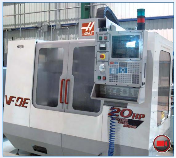
2000 HAAS CNC Lathe Model VF-OE, Travels: X-30", Y-16", Z-20", Table Size 30"x16", Cat 40, 7,500 RPM, Max Table Load 3,000 lbs, 20 HP, Rigid Tapping, 4th Axis Ready, Quick Code, Brushless Servos, sn 22839 (Dorion, PQ). View Video On Website!
