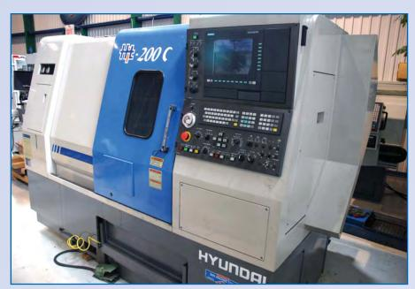
2004 **HYUNDAI** CNC Lathe Model HiT-200C, Distance Between Centers 13.78", Swing Over Bed 22.4", Swing Over Carriage 14.4", Travels: X-9.4", Z-16.9", 10" 3 Jaw Chuck, 10 Station Turret, Spindle Bore 3.15", Tailstock, Siemens 810D Sinumerik Controls, 36-3,600 RPM, Rapid Traverse 1,181 IPM, Cutting Feedrate 3,150 IPM, 20 HP, sn 1622D021 (Dorion, PQ)
