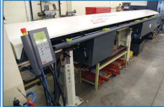
1999 **LNS** Hydrobar Express 226 Bar Feed, Set of 1-3/4" & 1-1/4" Pushbars & Guiding Channels Included, sn 100237 (Currently Feeding Hardinge)
