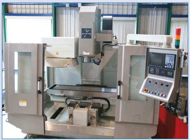
NEW 2008 HERCULES Heavy Duty VMC, Model BMC-5A, Mitsubishi 64-SM CNC Control, Travels: X-41-1/4", Y-22", Z-20-1/2", Table Size 16-3/4"x62", 10,000 RPM, Cat 40, 20 ATC, Max Table Load 1,320 lbs, Feedrate 197 IPM, 15 HP, 600V, sn 081057 (Dorion, PQ)
